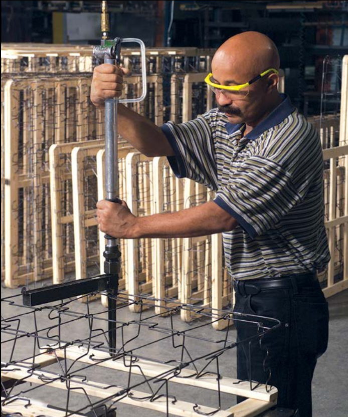
BCAR-2S Stapling foundation spring to flat
