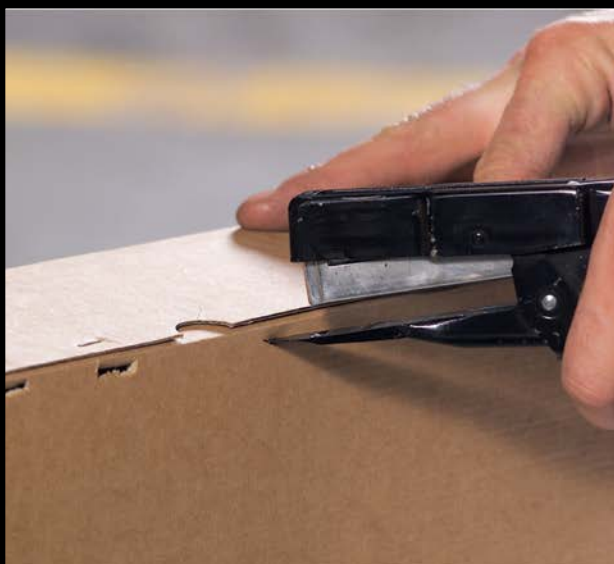
D62ADCSB With pointed anvil piercing corrugated to seal container from outside
