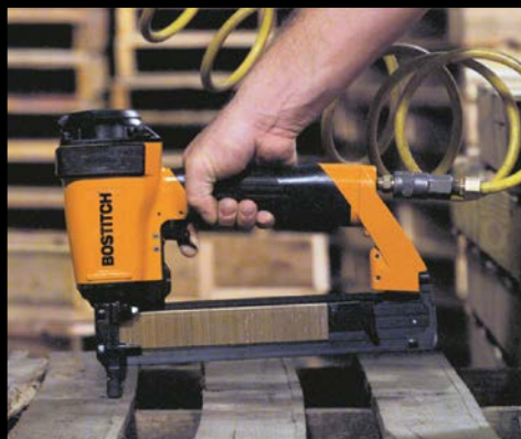
650S4-1 Reattaching Deck Board
