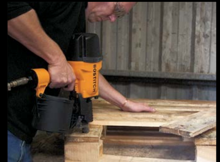
N400C-1* Nailing mat to block pallet
