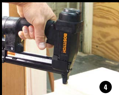
Caseback being secured with 18-gauge SL staples
