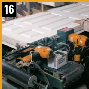
Machine mounted 750S4 Stapler equipped with remote TVA-4 trigger valves.
