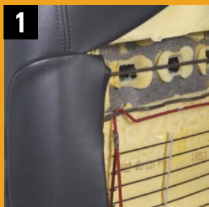
Automotive seating cover secured to frame with a 15-gauge C-ring. Back assembly fastened with clinch clip.
