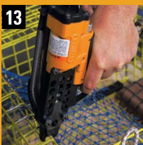
SC742 short magazine tool attaching pot head to cage frame
