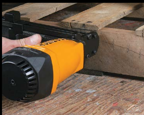
CF15-2 Pneumatic corrugated tool repairing split stringer
