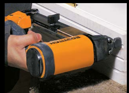
450S2-1 Stapler joining door jambs
