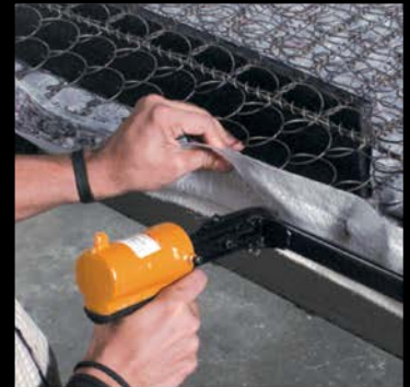
TR203 D-Ring tool connecting flange to innerspring
