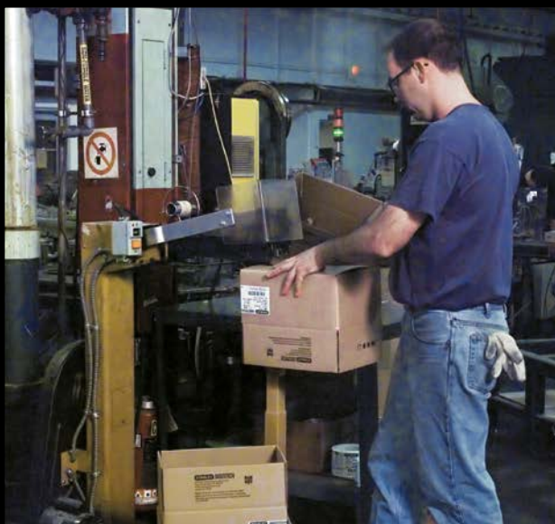
FC96EC Bottom closer used to clinch carton bottoms
